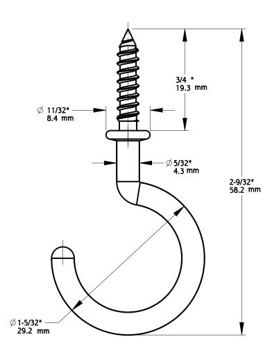
Material: Steel Fasteners: N/A
