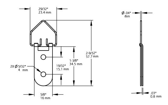
Material: Steel Finish: Zinc Plated Fasteners: Screws, #8x3/4" Pan(2 per)
