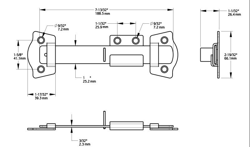
Quantity: 1 Fasteners: (6) #10 X 1-1/4" FH Type AB Tapping Screws Material: Steel Finish: Black
