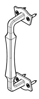
Fasteners: (4) #12 X 1-1/4" FH Type AB Tapping Screws Material: Steel Finish: Black
