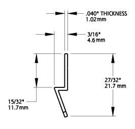
Material: (2)Aluminum Finish: Mill Fasteners: (2)#4X 1/2", FLAT HEAD, TAPPING SCREW (2)#8X 1", BEARCLAW HANGER, TAPPING SCREW
