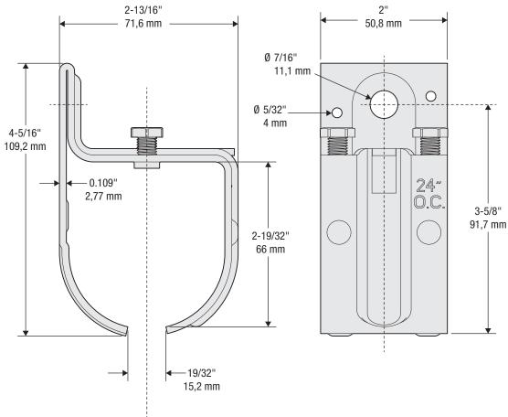
Each bracket installs with one 3/8"x2" Lag Screw at 24" maximum between bracket centers.
