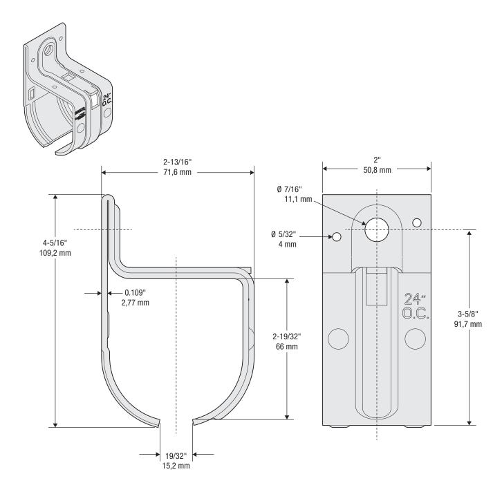
Each bracket installs with one 3/8"x2" Lag Screw at 24" maximum between bracket centers.
