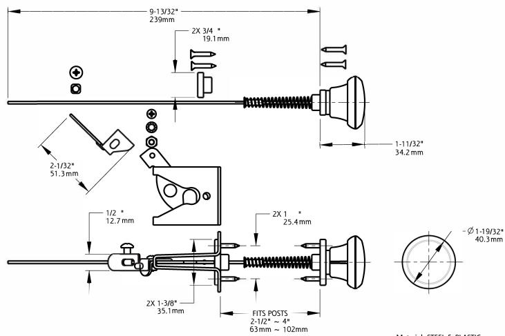
Material: STEEL & PLASTIC Finish: BLACK Fasteners:(4) #6X 3/4", FLAT HEAD, TYPE AB, TAPPING SCREW
