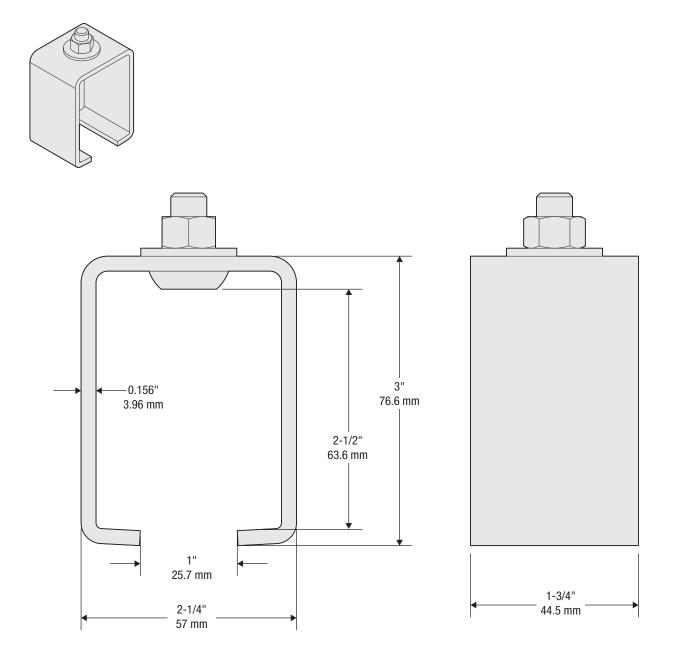
QPP: 1 Order Qty: 50 Material: Steel Finish: Zinc Fasteners: (1) Carriage Bolt, 3/8"-16 x 13/16", (1) Washer, (1) Nut
