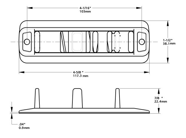
Material: PLASTIC & STEEL FINISH: YELLOW CHROMATE Fasteners: SCREW, PAN HEAD, #8X 5/8"
