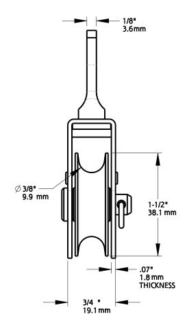
Material: Steel Finish: Zinc Plated Fasteners: (3) N/A
