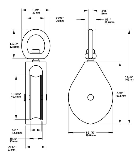
Material: Zinc Finish: Nickel Plated Fasteners: N/A
