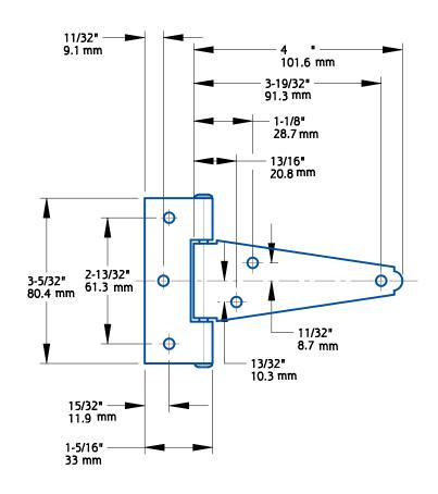
Material: Steel Fasteners: (6) #9 X 3/4", Type AB, FH, Full Thread, X-Rec, Screw
