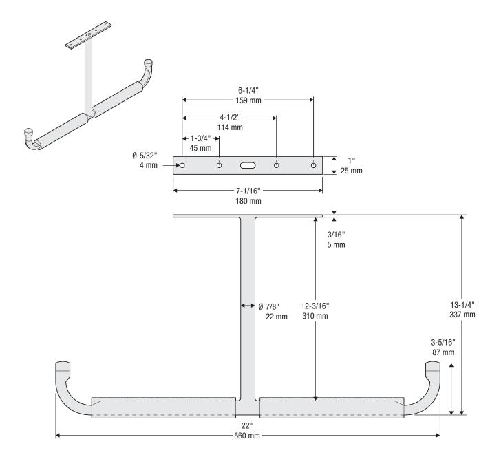
Material: Steel Finish: Gray Powder Coating SWL: 50 lbs Fastener: (2) #10-16 x 2" Long Type A, Phillips, Round head Pilot hole: 1/8"
