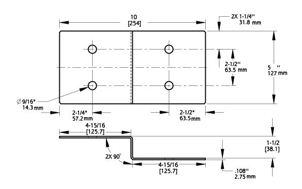
Material: Steel Finish: E-coat + black powder coat Fasteners: N800-022 = 1/2" x 3" or equal
