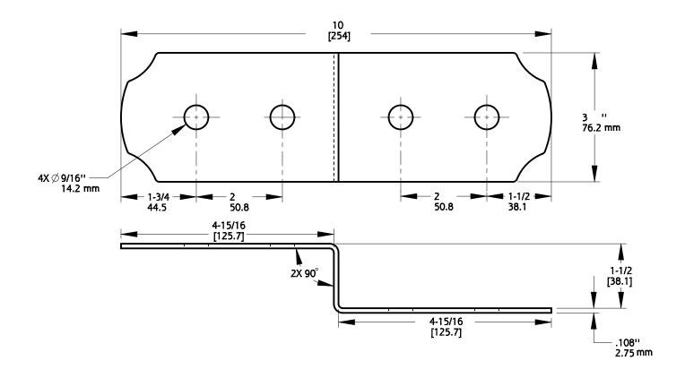
Material: Steel Finish: E-coat + black powder coat Fasteners (not included): N800-123 = 1/2" x 1-1/2" lag or equal
