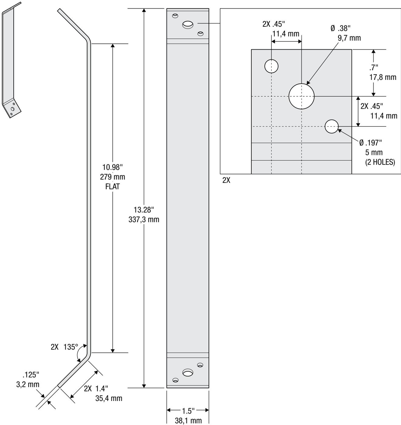
Hole Information: Clearance for 5/16" bolt or 2 nails per side
