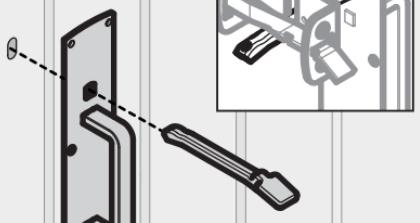
Toggle thumbpiece while inserting to secure.
