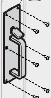
Before securing, hold down thumbpiece to ensure it can completely lift the latch to open gate.
